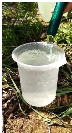
(b) Mine water pumped by a submersible pump from a depth of 3 m below the surface
