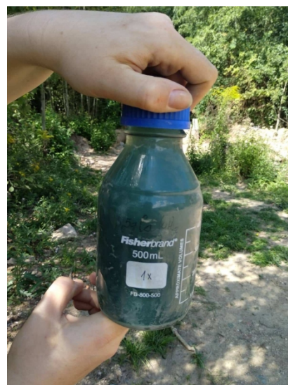
(c) Mine water after mixing with \text{Ca}(\text{OH})_2 . Formation of blue-green ferric hydroxide precipitate
