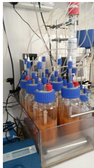
Fig. 5. Laboratory tests of chemical and bacterial oxidation of iron in mine water with online analysis of gases, pH and ORP.
